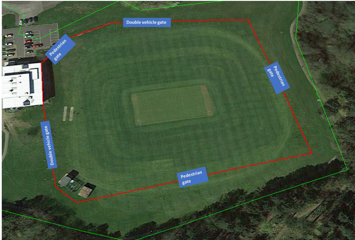
Figure 2: proposed perimeter of fencing and illustration of gate positions (the exact perimeter line and gate positions to be agreed with the contractor prior to works commencing)
