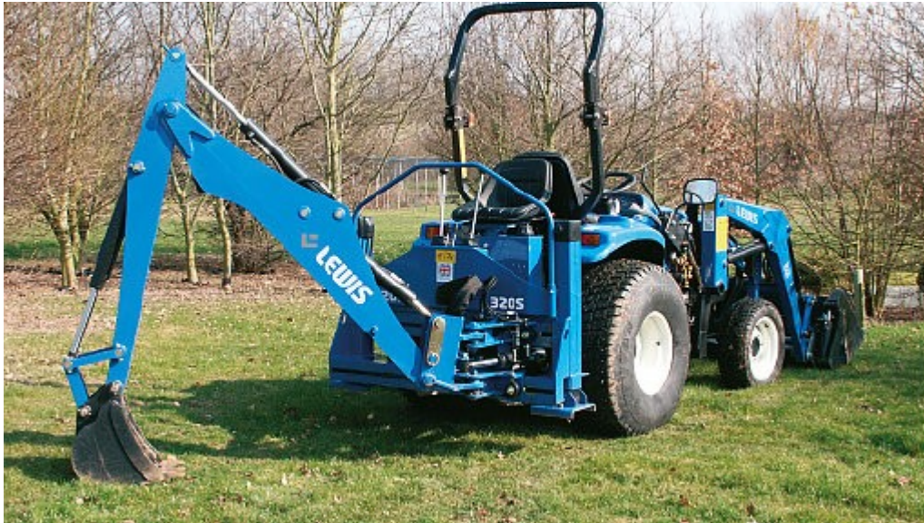
Figure 3: Lewis 320 s backhoe
